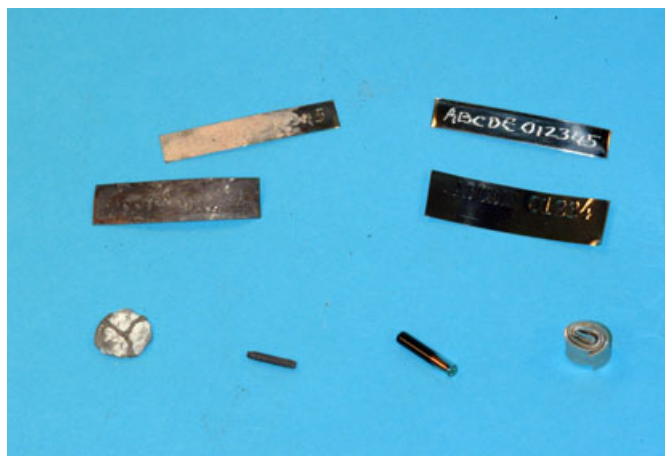
FIG. 2—Remains of the fire experiment, i.e., the stainless steel orthodontic band, the ID-Band, the soft metal foil, and the remains of the RFID-tag. Featured on the right are the intact versions of the labels.
