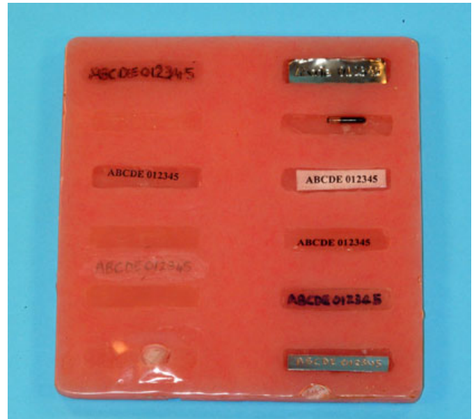
FIG. 1—A 10 × 10 × 0.5 cm block manufactured from polymethylmethacrylate acrylic (PMMA) pink/veined denture base resin. One example of each denture identification label was placed into the block to a depth of 2 mm before being covered by clear self-cure PMMA.
